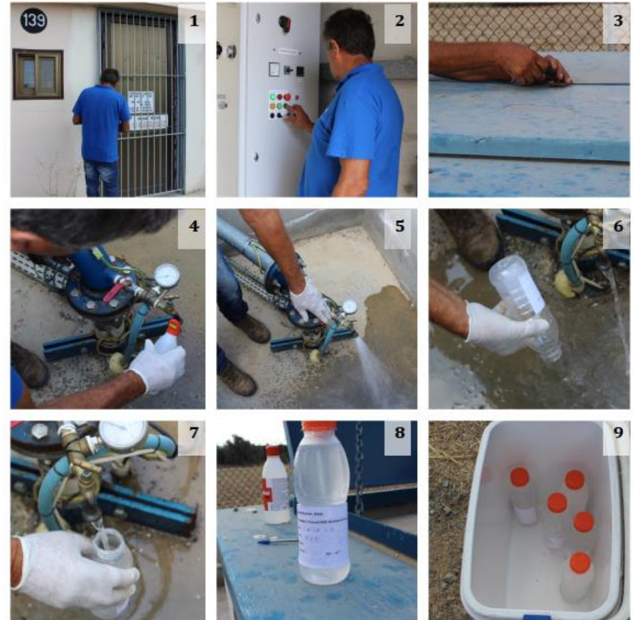
Figure 3.1: Water Sample Collection for WSBA boreholes (BH1-BH3)
